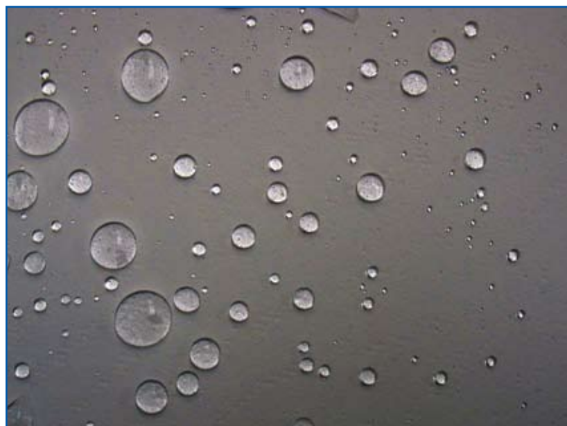
Figure 10: Hydrophobic surfaces cause water to bead, minimizing impact to RF performance under wet conditions.
